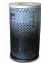
Fuel filter after 12,000 miles using typical #2 diesel.
